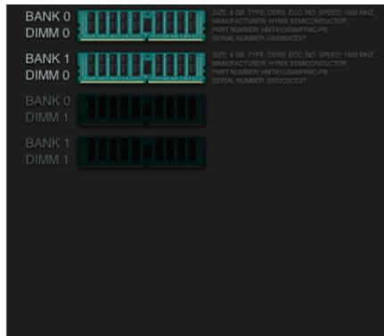
along with available slots. The DIMM addresses are listed to the left of the modules, and the text to the right describes the installed module.
